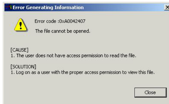
Fig. E.1 This Error Message is Displayed If an Attempt is Made to Open a User Application (i.e., ladder, motion, or C language).
